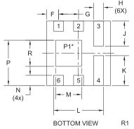
\*Exposed pad P1 common to pins 1, 2, 5, and 6.
